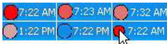
Figure 3 Virtual Intimate Object (VIO) in taskbar, showing color changes over a twelve hour period. Note rapid initial fading in top line. Final image shows display of remote partner’s button state on mouseover.
